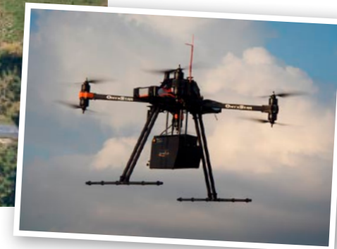
▼ The YellowScan laser scanner system on board an octocopter.
